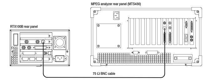
Figure 3-8: Equipment connection for checking the recorded file- ASI interface
