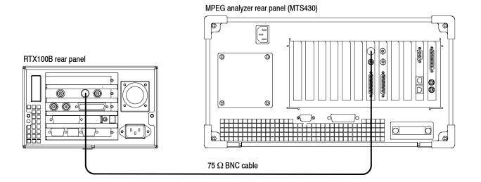
Figure 3-7: Equipment connection for checking the record operation- ASI interface
