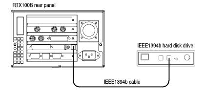
Figure 3-13: Equipment connection for checking the IEEE1394b interface
