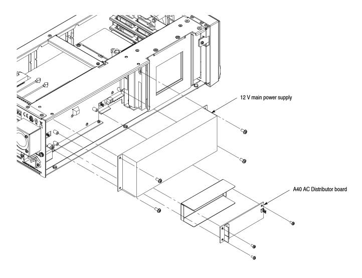
Figure 5-13: 12 V main power supply and A40 AC Distributor board removal
