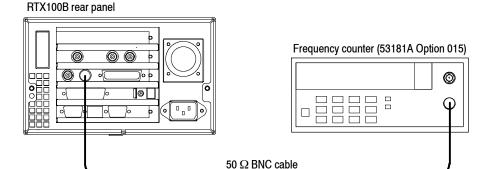
Figure 3-2: Equipment connection for checking the internal clock frequency
