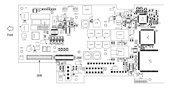
Figure 5-24: A20 PCI Backplane board view-right side
