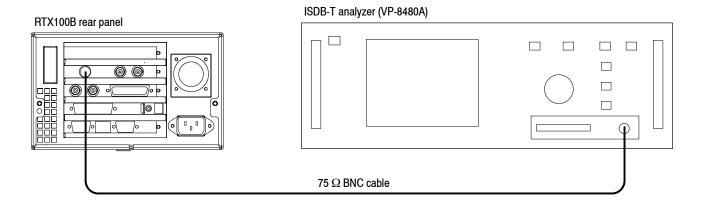
Figure 3-12: Equipment connection for checking the output level and error
