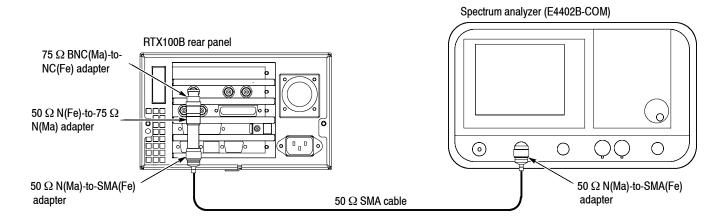
Figure 3-11: Equipment connection for checking the carrier leakage
