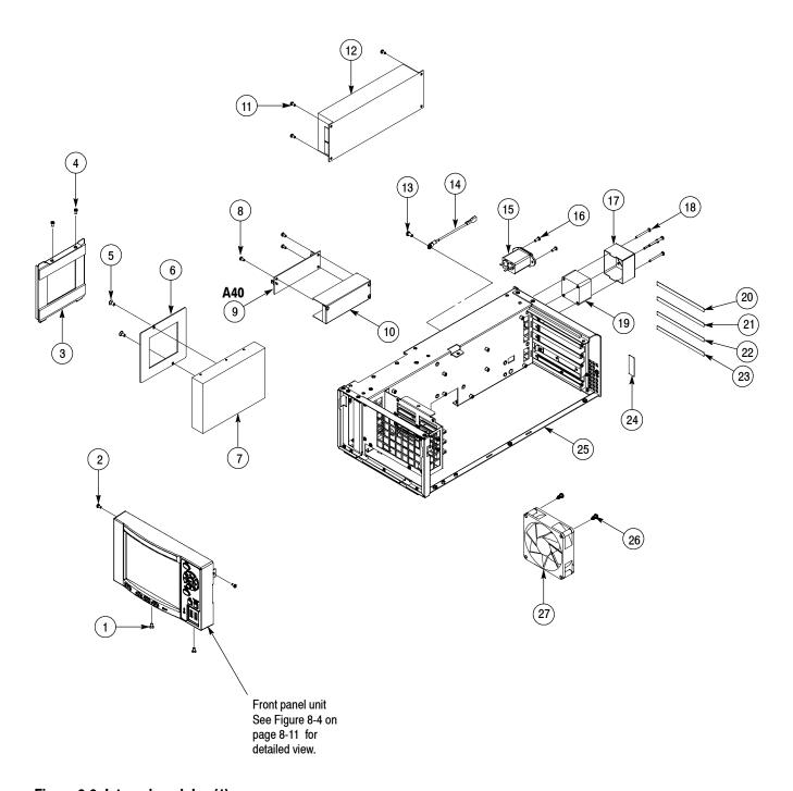
Figure 8-2: Internal modules (1)
