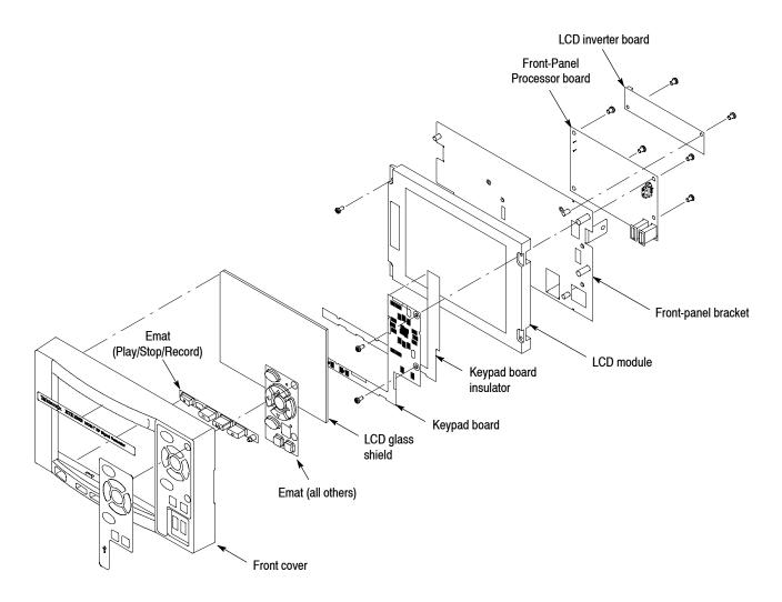
Figure 5-9: Disassembly of front-panel assembly
