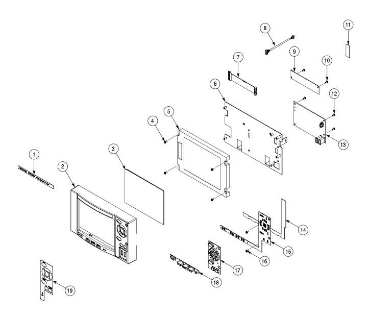
Figure 8-4: Front panel unit
