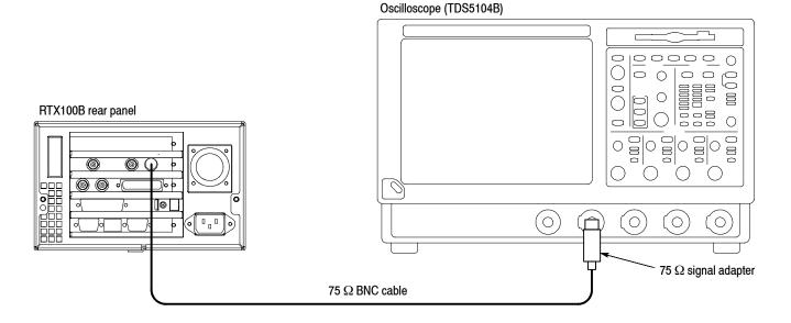
Figure 3-5: Equipment connection for checking the output signal-ASI interface
