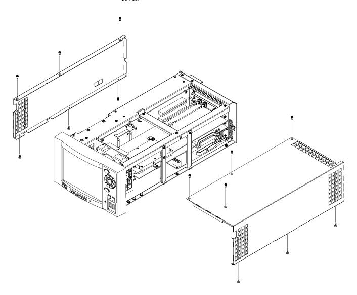
Figure 5-7: Right-side and left-side covers removal
