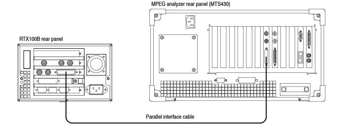
Figure 3-3: Equipment connection for checking the play operation-SPI interface
