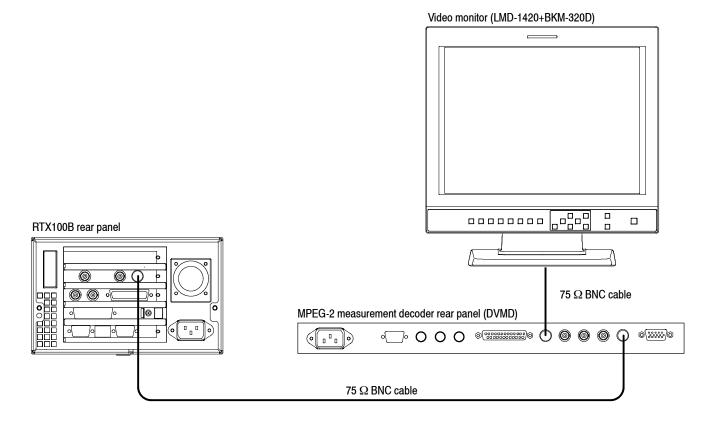
Figure 3-9: Fifth equipment connection for checking the ASI interface
