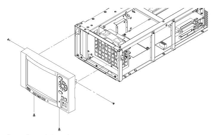
Figure 5-8: Front-panel unit removal
