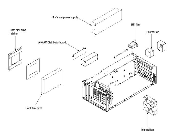
Figure 5-4: Internal modules
