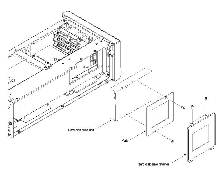
Figure 5-11: Hard disk drive removal
