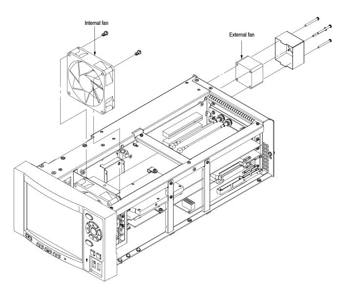
Figure 5-12: Internal and external fan removal
