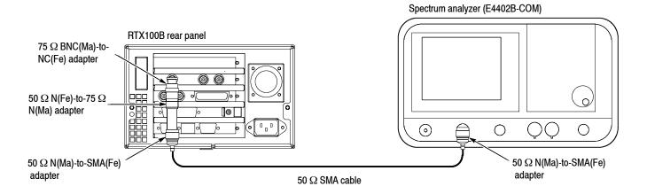
Figure 4-1: Equipment connection for adjusting the carrier leakage
