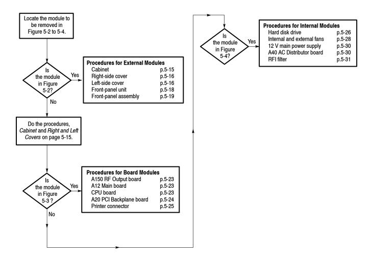
Figure 5-5: Guide to removal procedures
