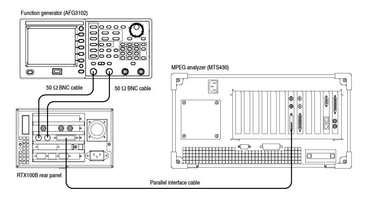
Figure 3-4: Equipment connections for checking the external clock/reference and trigger inputs
