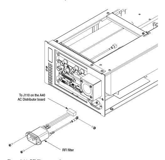
Figure 5-14: RFI filter removal
