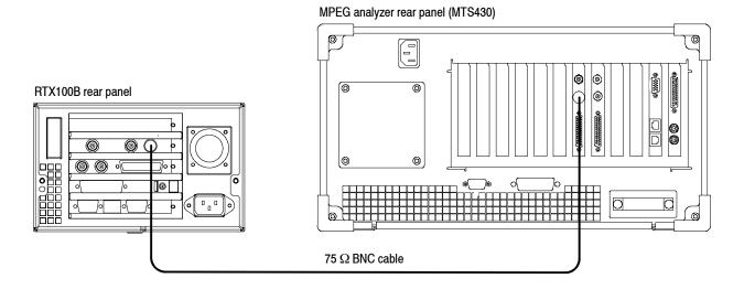
Figure 3-6: Equipment connections for checking the play operation-ASI interface
